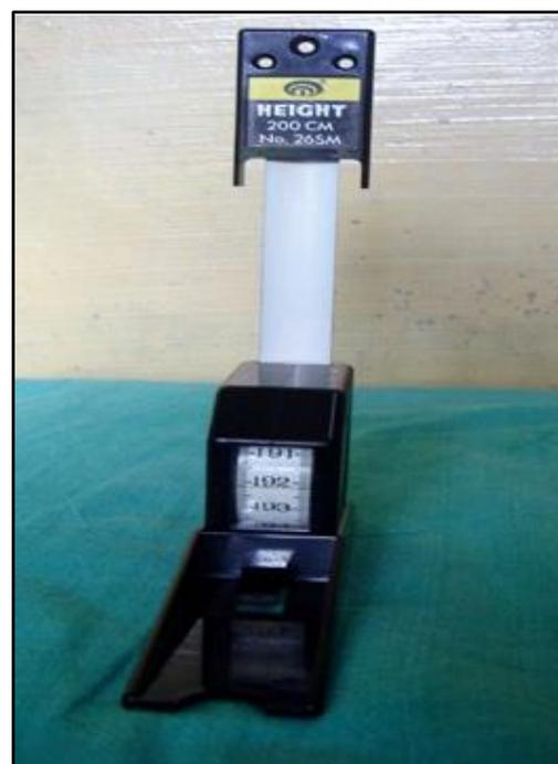
**Figure 2. Sliding Stadiometer (Johnson and Johnson)**
