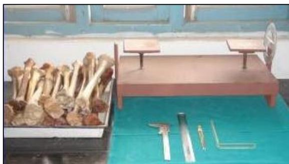
**Figure 1. Specimens, Self-Designed Osteometric Board and Equipment**
