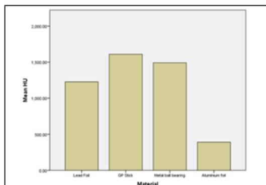
**Figure 2. Bar graph showing the mean Hounsfield units for each of the material from the different exposure protocols.**
