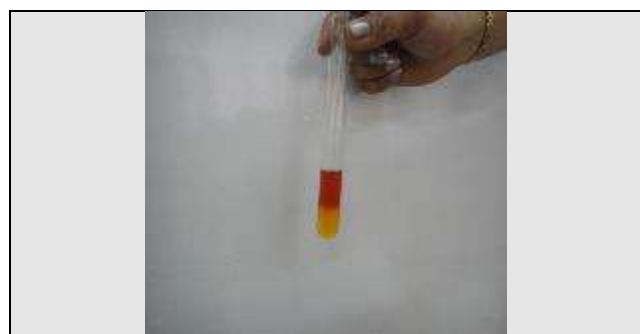
Picture 1. Nitric Acid Test: 5 mL Oil is Shaken with an Equal Volume of Nitric Acid. On Standing, the Acid Layer Turns Yellow, Orange-Yellow or Crimson, Depending Upon the Amount of Argemone Oil. The Test is Sensitive to a Concentration of >0.25%.
